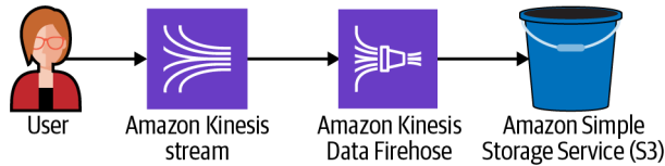
Figure 7-2. Streaming data to Amazon S3 using Amazon Kinesis Data Firehose
